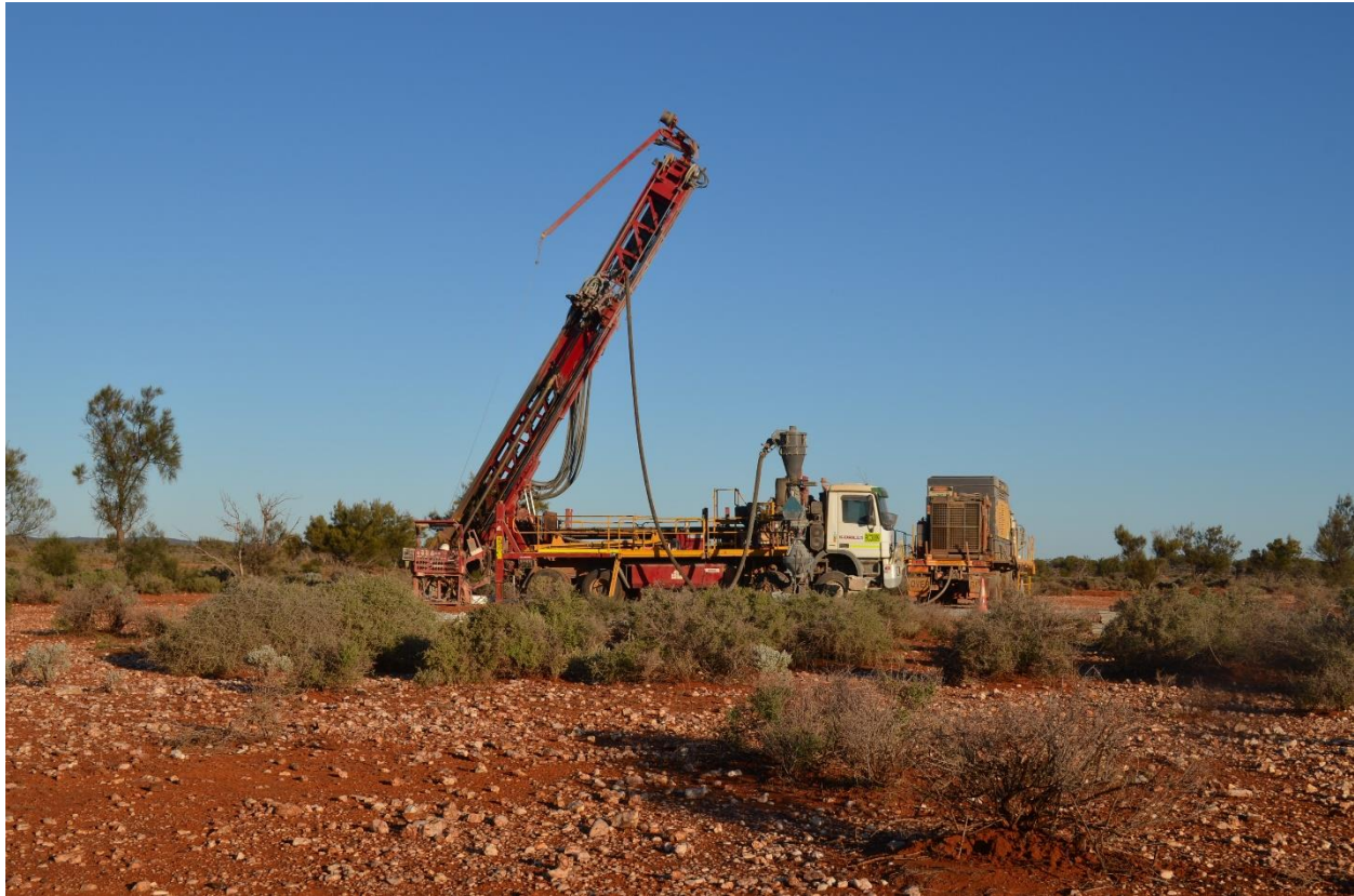
Figure 2. K-Drill RC rig drilling at the Red Gate Gold Project
