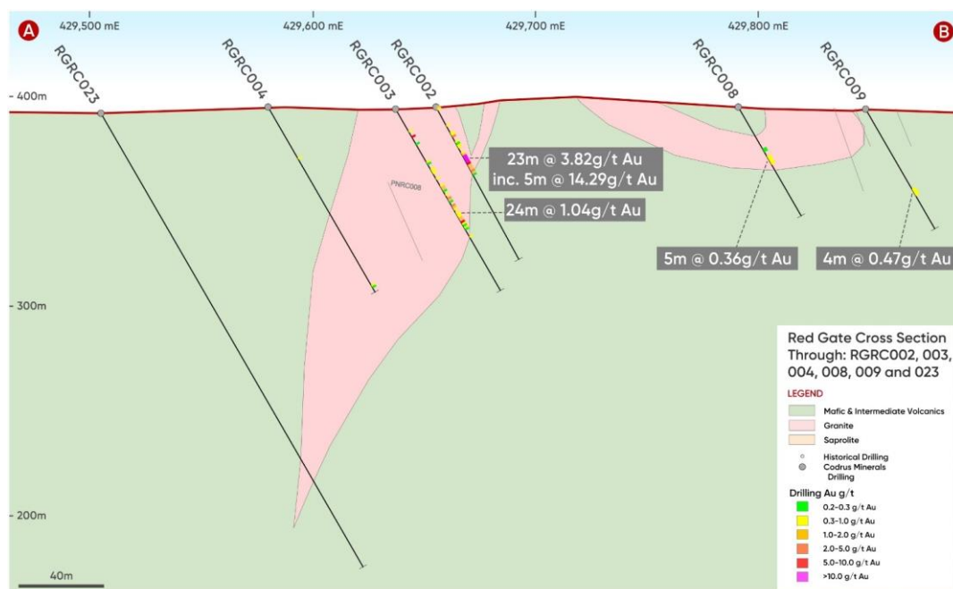
Figure 5. Cross section through Porphyry West showing the mineralisation in RGRC009, 002, 003, 004, 008, 009 and 023.
