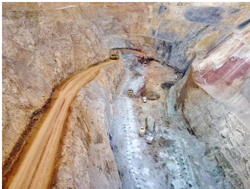
Figure 1: Zoroastrian Central Open Pit looking South (mining on the 345 to 342.5mRL). Mining is planned to the 320mRL.
