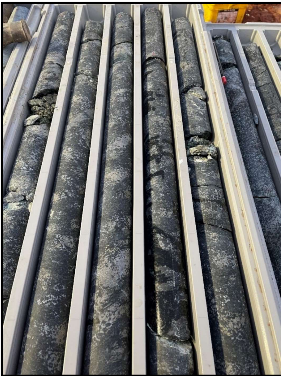
Photo 4: High MgO ultramafic encountered in RKDD059 from 346m from the new intrusion 2km south of Mawson.
