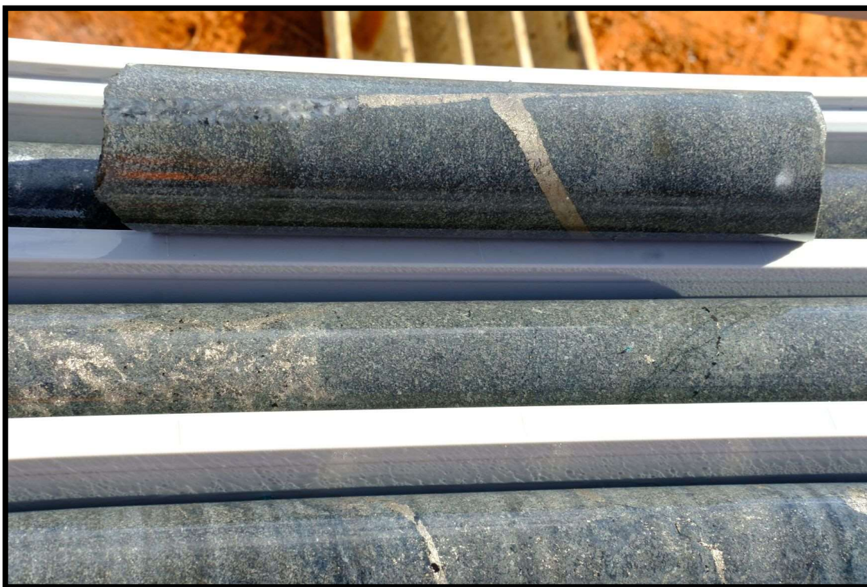
Photo 3: Ni-Cu sulphide mineralisation from RKDD062.
