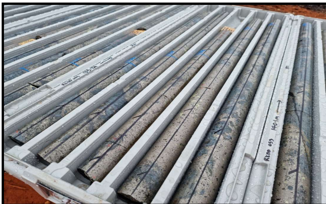
Photo 1: Ni-Cu sulphide mineralisation from RKDD053 from 135-140m.
