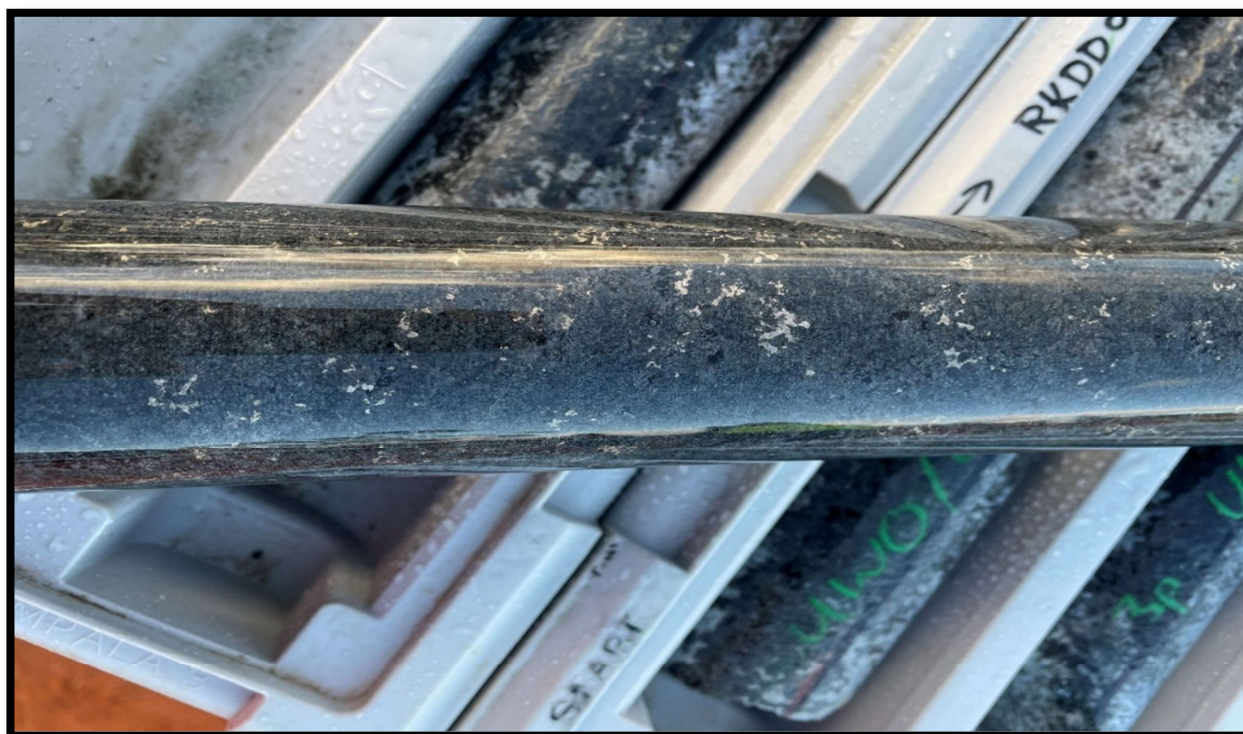
Photo 2: Disseminated Ni-Cu sulphide from RKDD058 from 320m.
