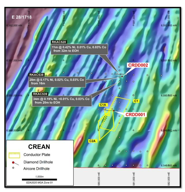
Figure 2: Crean Prospect showing drilling completed over aeromagnetics
