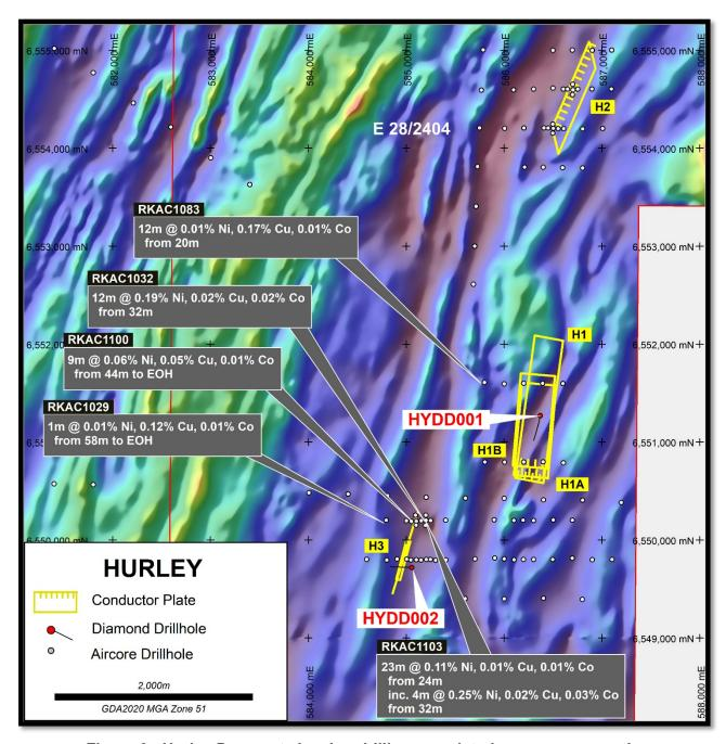
Figure 3: Hurley Prospect showing drilling completed over aeromagnetics
