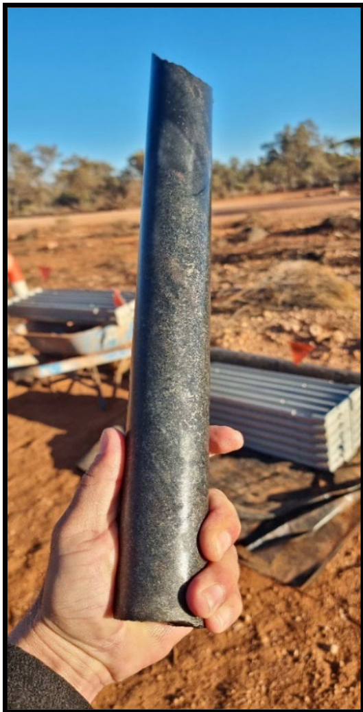
Photo 1: Heavy disseminated sulphide intrusion from RKDD081 from 840m, NQ2
