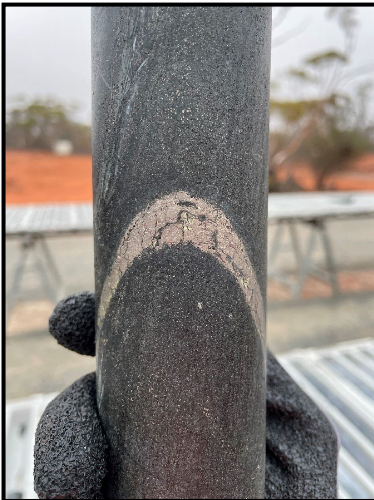
Photo 2: Cross-cutting massive sulphide vein from RKDD082W1 from 819.3m, NQ2
