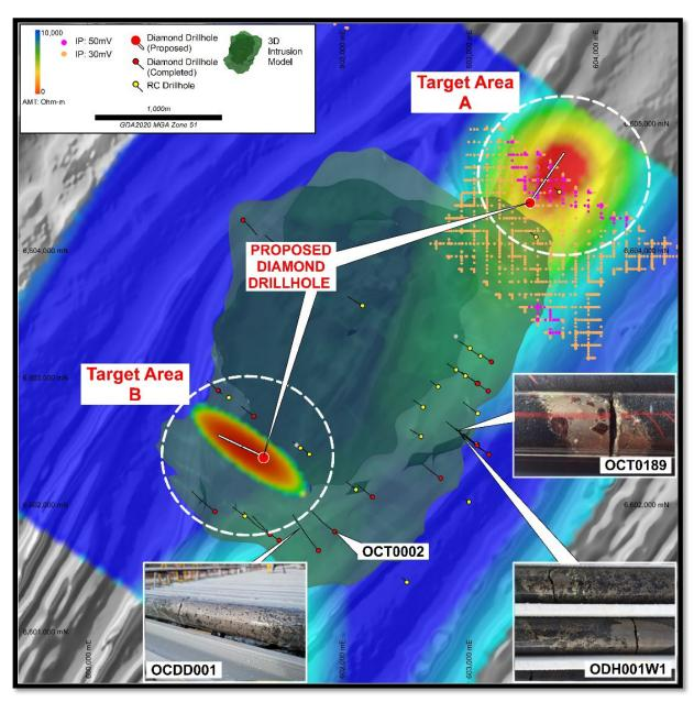
**Figure 1:** Priority target areas and proposed diamond drillholes shown with Octagonal intrusion model, IP anomalies, 2D & 3D AMT anomalies and existing drilling with visual Ni-Cu mineralisation on AMAG.
