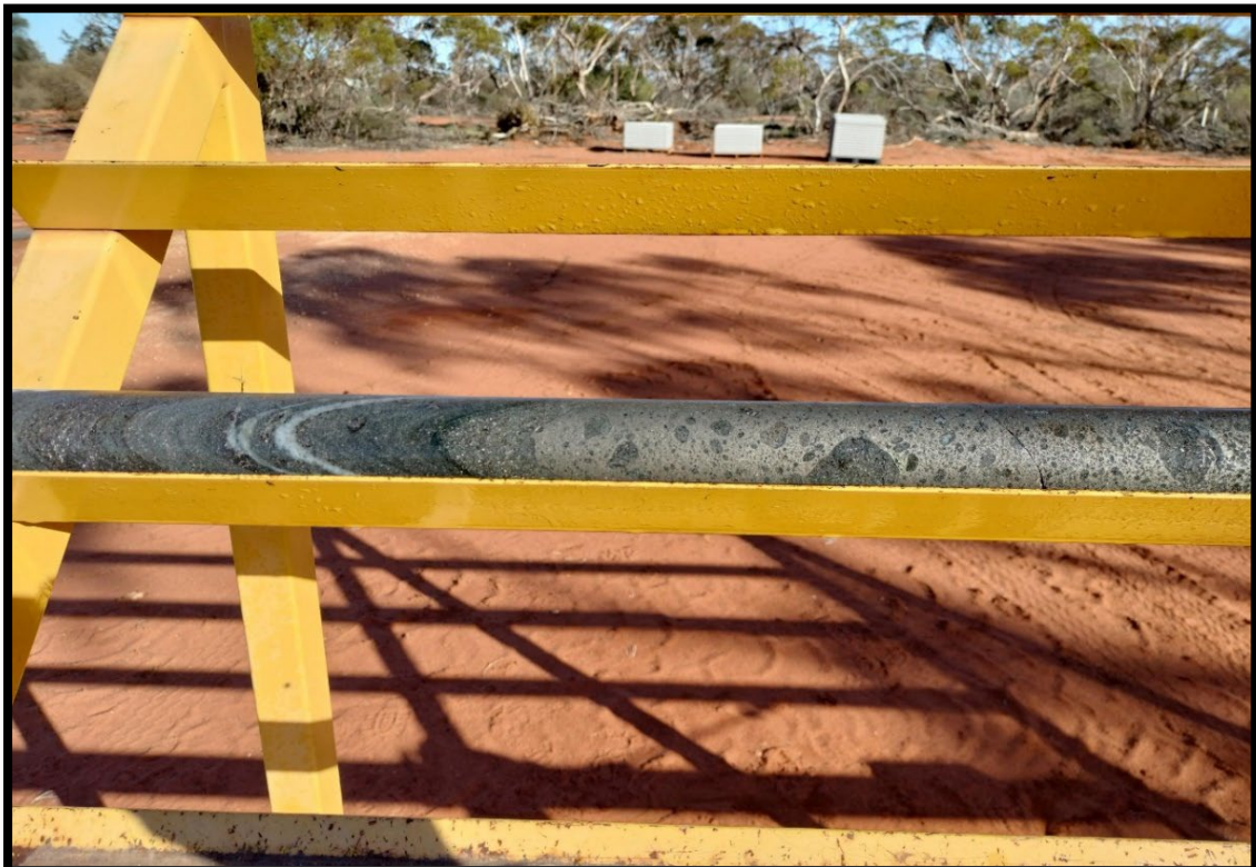
Photo 1: Semi-massive, brecciated Ni-Cu sulphide from diamond drillhole OCDD003 from 501m.
