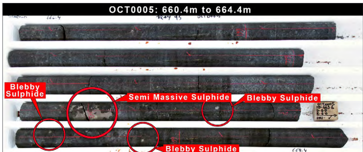
Photo 3: Diamond drill core tray from OCT0005 with visual Ni-Cu sulphide mineralisation. OCT0005 intersects the top edge of conductor 2.
