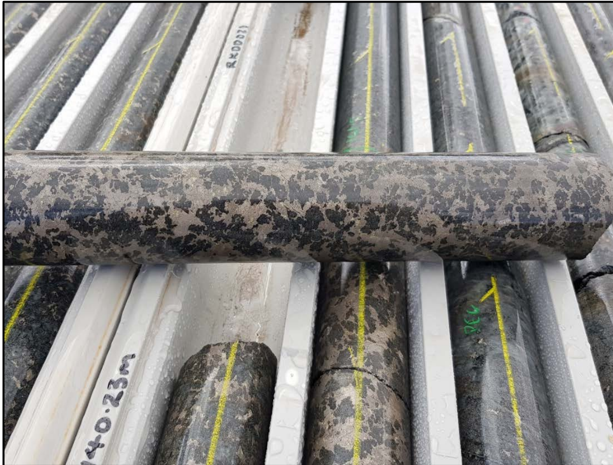
Net-Textured Ni-Cu Sulphide mineralisation from RKDD021 from 140.5m, NQ2
