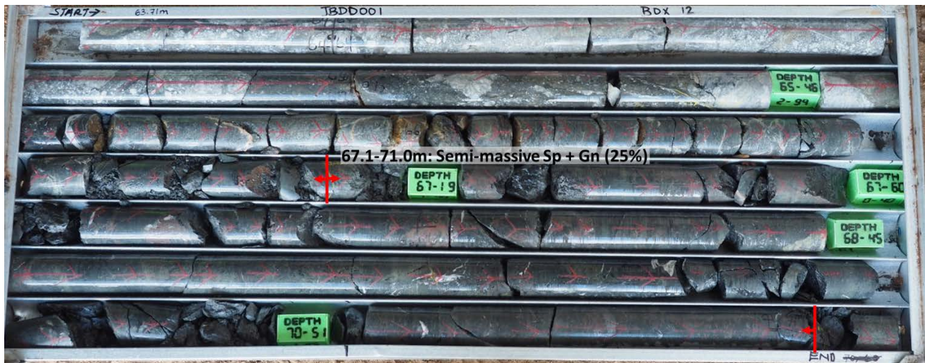
Figure 5. JBDD001 Semi-massive sulphide intersection containing approx. 25% total sulphides (sphalerite + galena), based on visual estimation of sulphide in ore.
