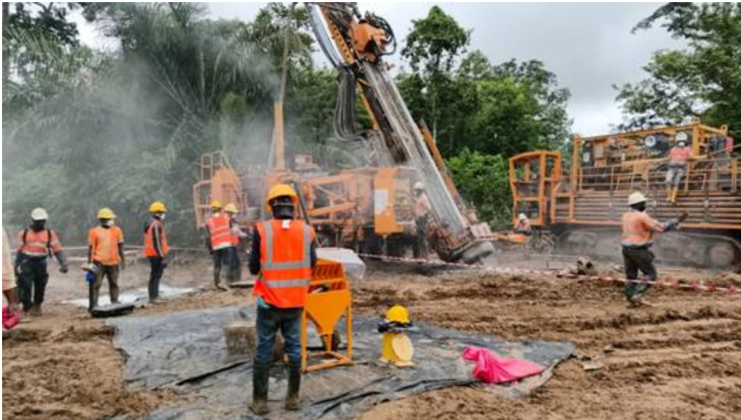
Photograph 2: RC drilling underway at the Zraty tantalum target, Issia Project, Côte d'Ivoire
