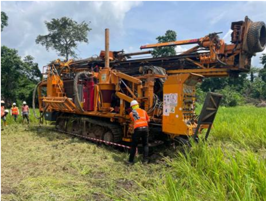
Photograph 2: RC drilling underway at the Zraty tantalum target, Issia Project, Côte d'Ivoire
