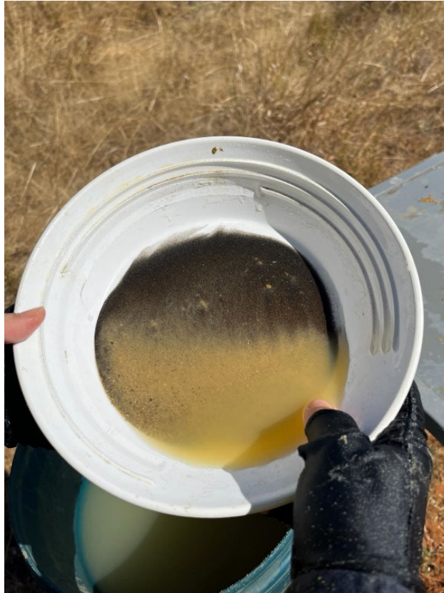
Figure 3 – Pan sample from 24m depth in drill hole 24DAC014, logged as Very High THM (>10%)
