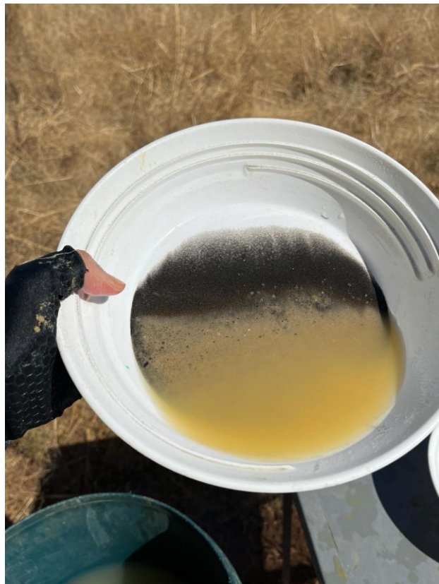
Figure 4 - Pan sample from 25.5m depth in drill hole 24DAC014, logged as High THM (7-10%)
