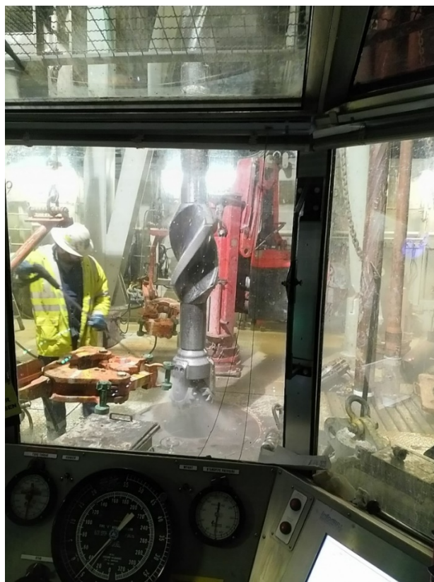
Figure 2: Pulling the 17 ½ inch bit assembly from the hole on the drill floor of the RED E-200 rig
