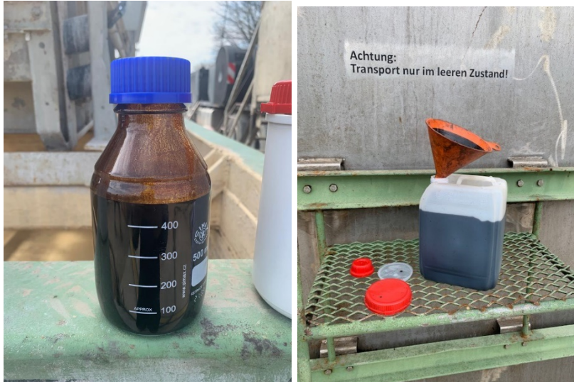
Sample of water free 36 API oil collected from Anshof-3 well flow test. Source ADX
