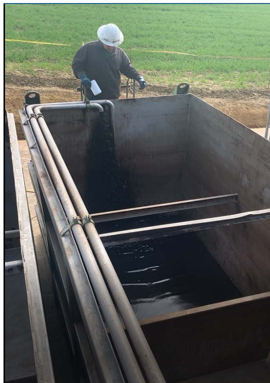
Oil production collected at surface during the Anshof-3 well flow test. Source ADX
