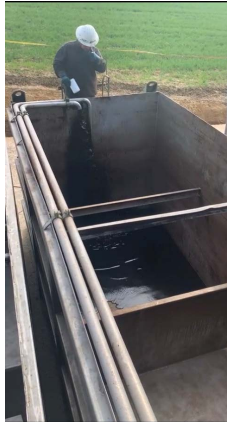
First oil flow to surf during testing High quality 33 API oil produced
