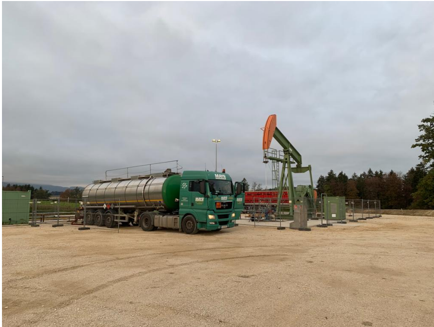
Figure 7: Oil tanker loading during long term testing at the Anshof-3 location
