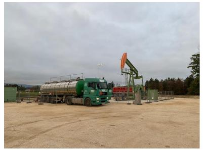
Fast-tracked early production using leased facilities, oil trucked to terminal for rail transfer to OMV refinery
