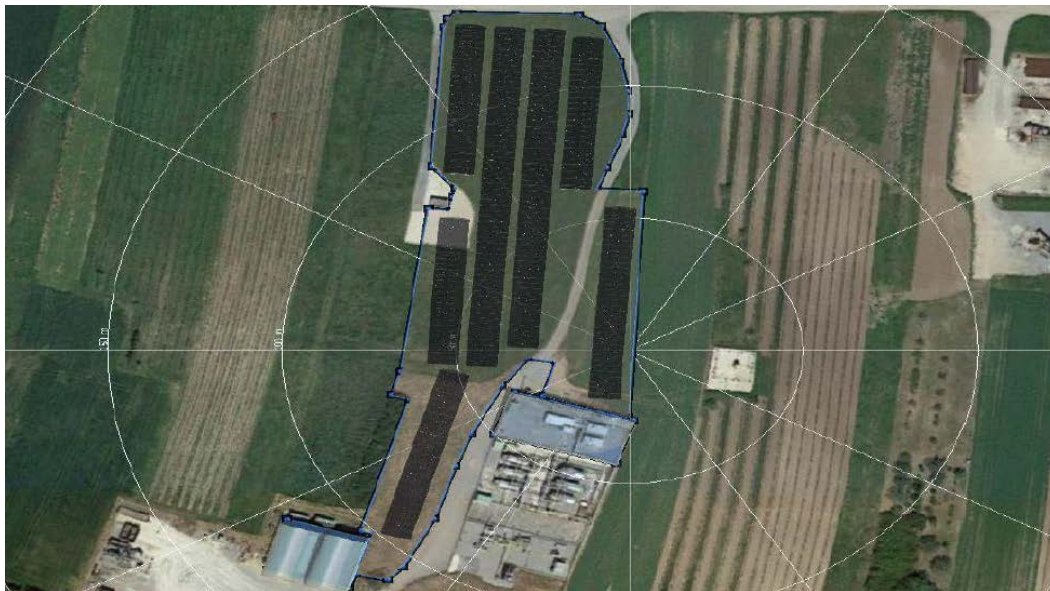
Figure 7: Potential layout of the PV panels at the Gaiselberg site (approx. 1 MWp)
