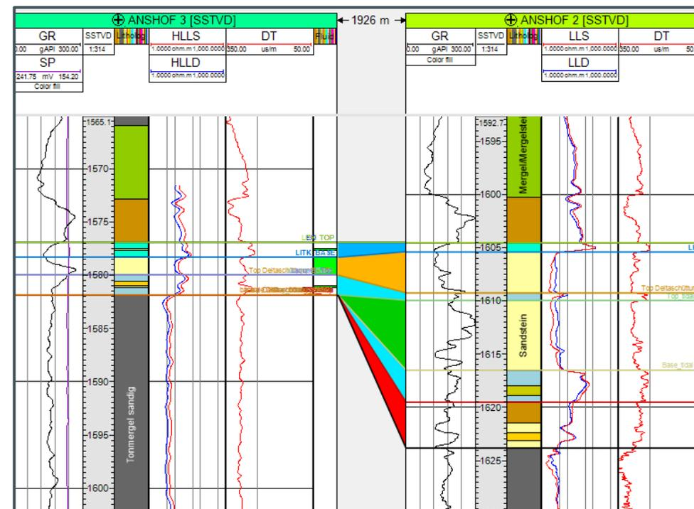
**Anshof-2 Sidetrack up-dip** likely to be next producer, replacing planned crestal ANS-1 producer and minimising well cost using existing ANS-2 well and sidetracking below existing 9 5/8” casing shoe.
