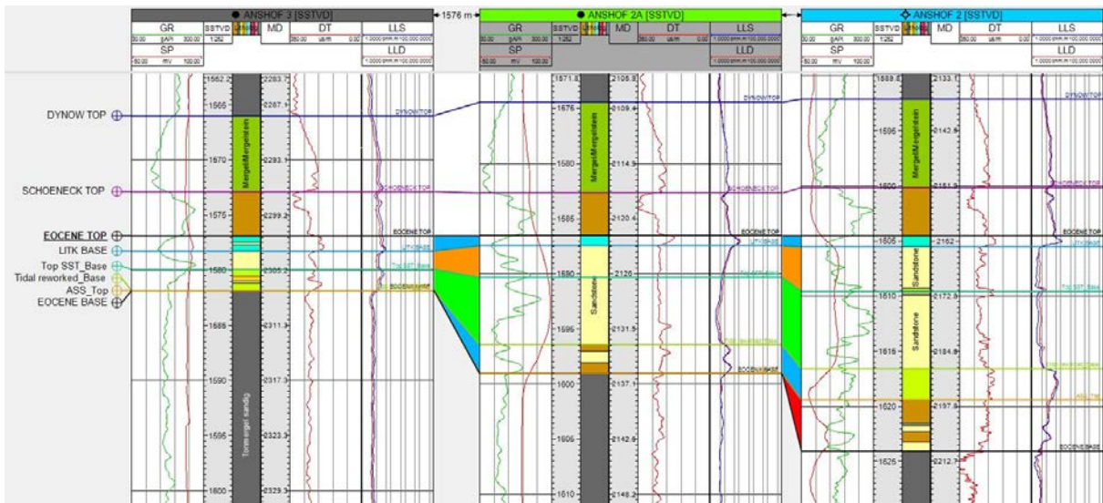
Figure showing a comparison of the Eocene sand thickness (shown in yellow) encountered in the Anshof-3 well (LHS), the ANS-2A well (Middle) and the Anshof-2 well (RHS)
