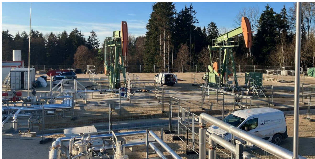
Figure 1: ANS-3 producing well and the recently installed ANS-2A well (on the right hand side) which has recently commenced production into the Anshof permanent production facility
