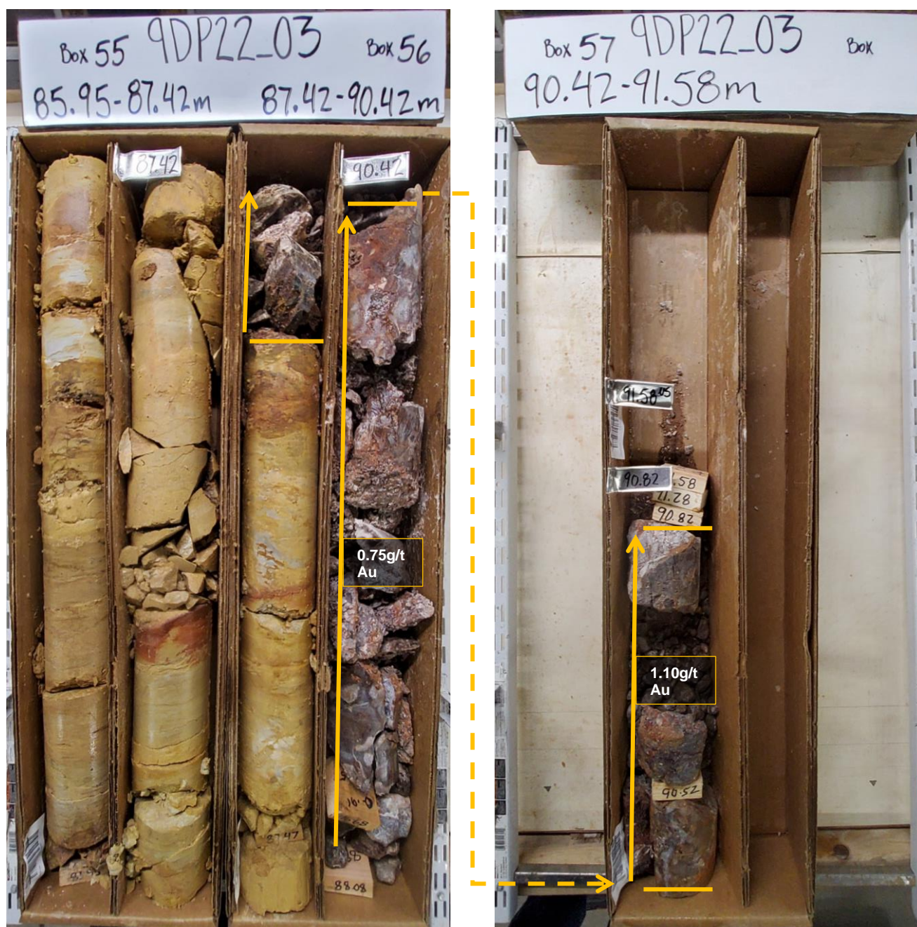
Figure 4: Photograph series of mineralised drill core from the hole 9DD22-003 with gold assays from 88.0 - 105.77m down hole. The overall mineralised intercept is 17.77m @ 1.70g/t Au which includes a 0.76m cavity grading 0.0g/t Au.
