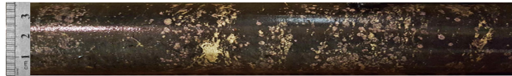
Photo of 36mm diameter Diamond Drill Core - Mineralisation style encountered in drill hole GRO20-02 at Green Mile. Biotite-Garnet-Amphibole alteration with 1-5% including visual chalcopyrite and minor pyrite, at 33.1m metres down 1 .
