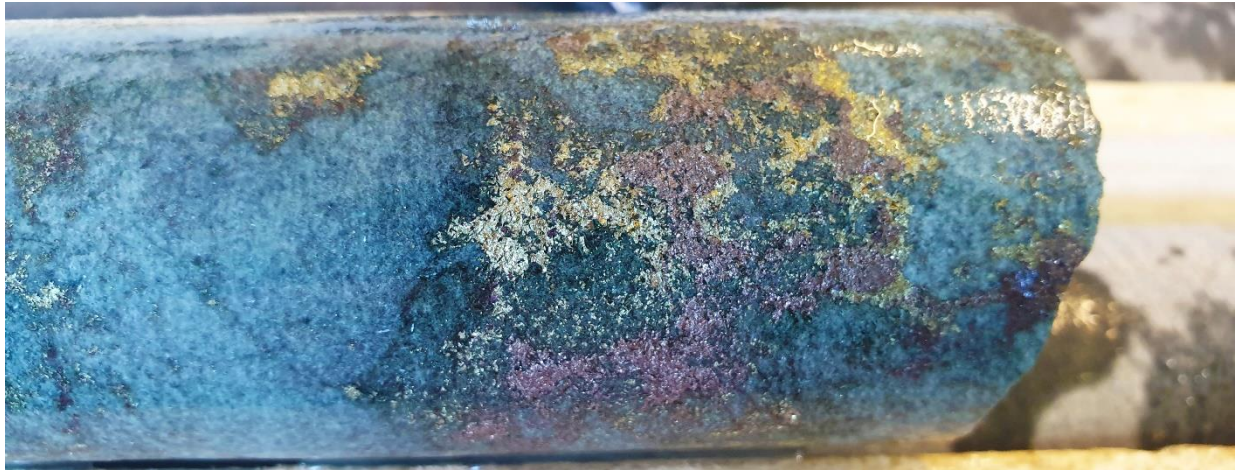
Photo 3: Drill core HED20-01 from 71.44m with visual sulphides of Chalcopyrite (visuals reported ASX:10/1/2020)
