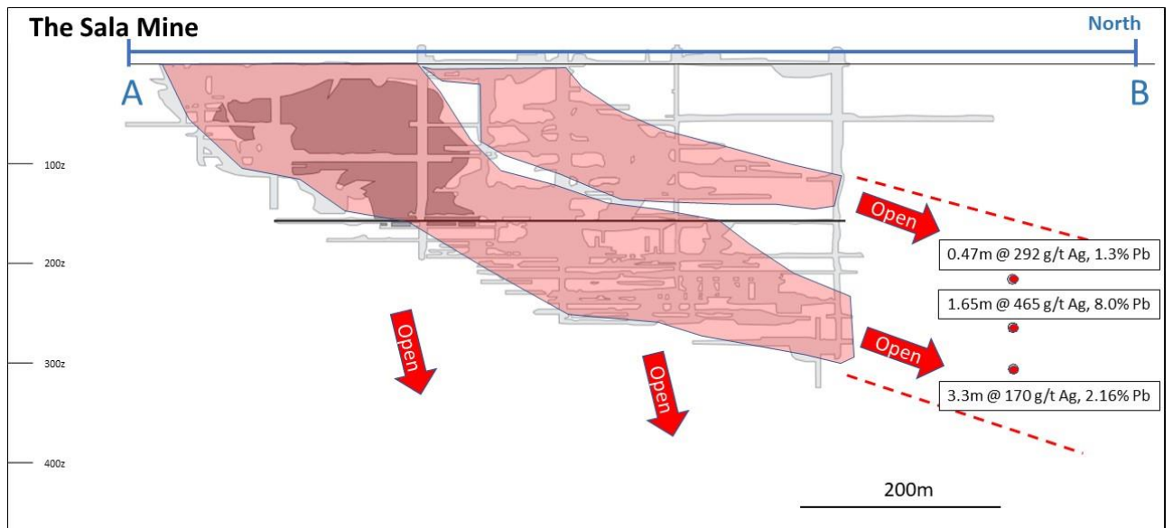
Figure 15: Long section of the Sala Silver mine looking west.
