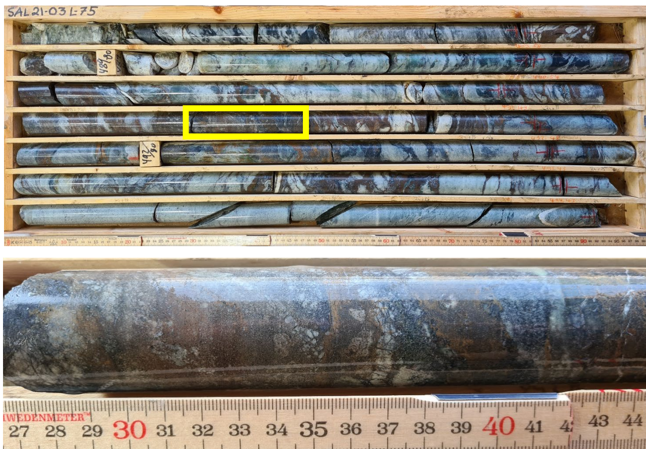
Figure 5: Visual intercepts from SAL21-03, showing the semi-massive zone of sphalerite-galena mineralization encountered from 489.58m to 494.43m.
