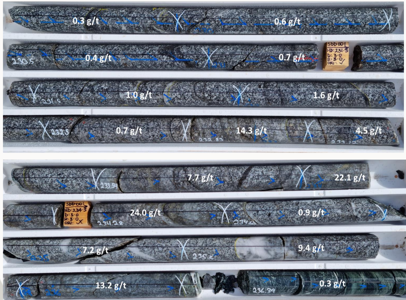
Lord Nelson diamond core from 229.6m to 236.8m showing strong sulphide rich alteration (SDD001).
