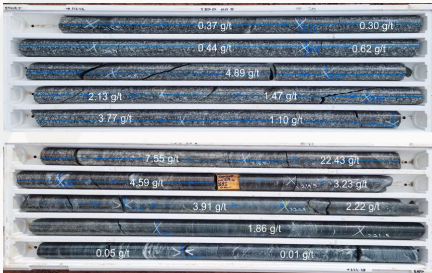
Lord Nelson NQ (47.6mm) diamond core from 213.42m to 222.58m showing high-grade gold mineralisation in strong quartz-pyrite veining, along the contact between silicified granodiorite and strong foliated ultramafic contact. SDD008
