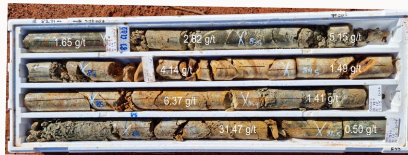
Orion Lode HQ3 (63.5mm) diamond core from 82.71m to 86.7m showing high-grade gold mineralisation in oxide and transitional zone. SDD008.
