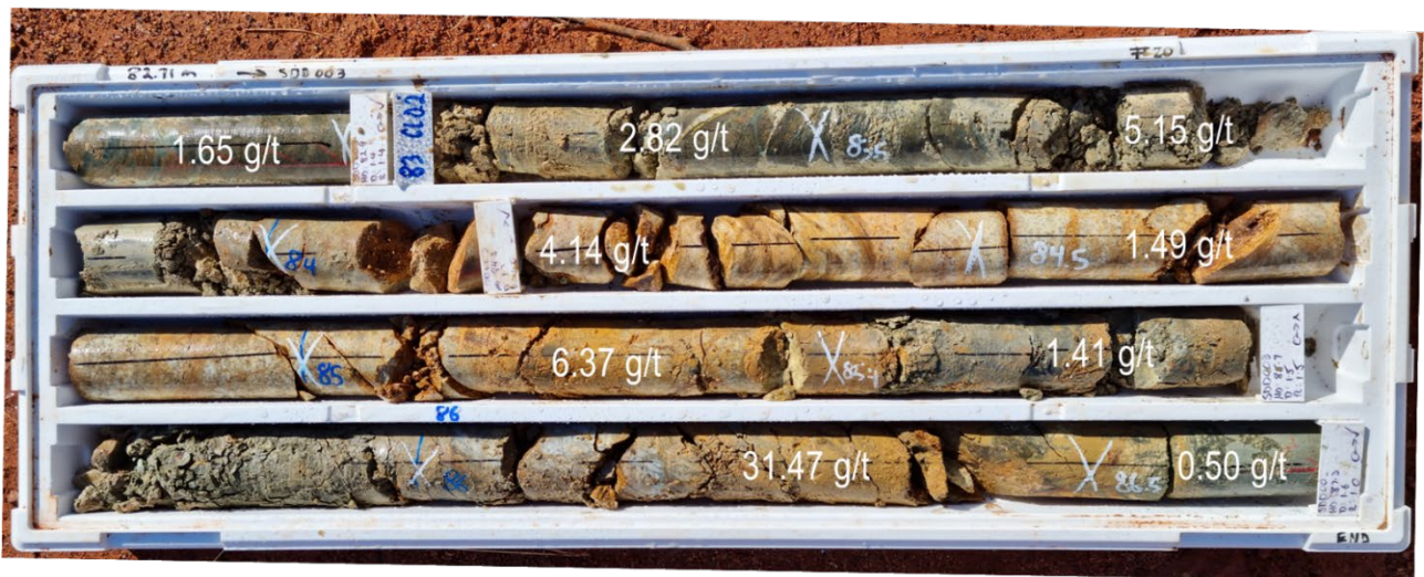
Figure 5: (SDD003) -Orion Lode HQ (63.5mm) diamond core from 82.71m to 86.7m showing high-grade gold mineralisation in oxide and transitional zone.
