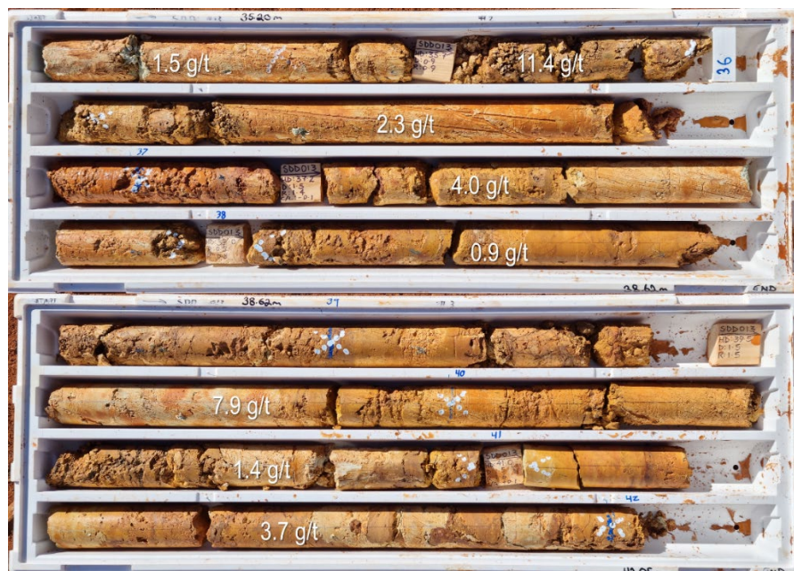
Figure 10. Diamond core from SDD013 from 35.20m to 42.05m HQ (63mm diameter). (Table above) Summary assay table for SDD013 from 29.4m to 49m
