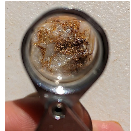
Above image: VG is RC chip from SRC918 from 29-30m interval assaying 122.6g/t gold (10x mag.)
