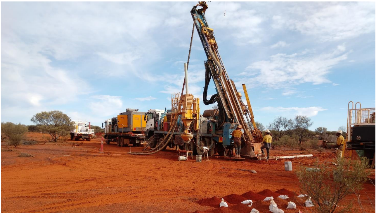
Figure 9: RC drilling at Indomitable
