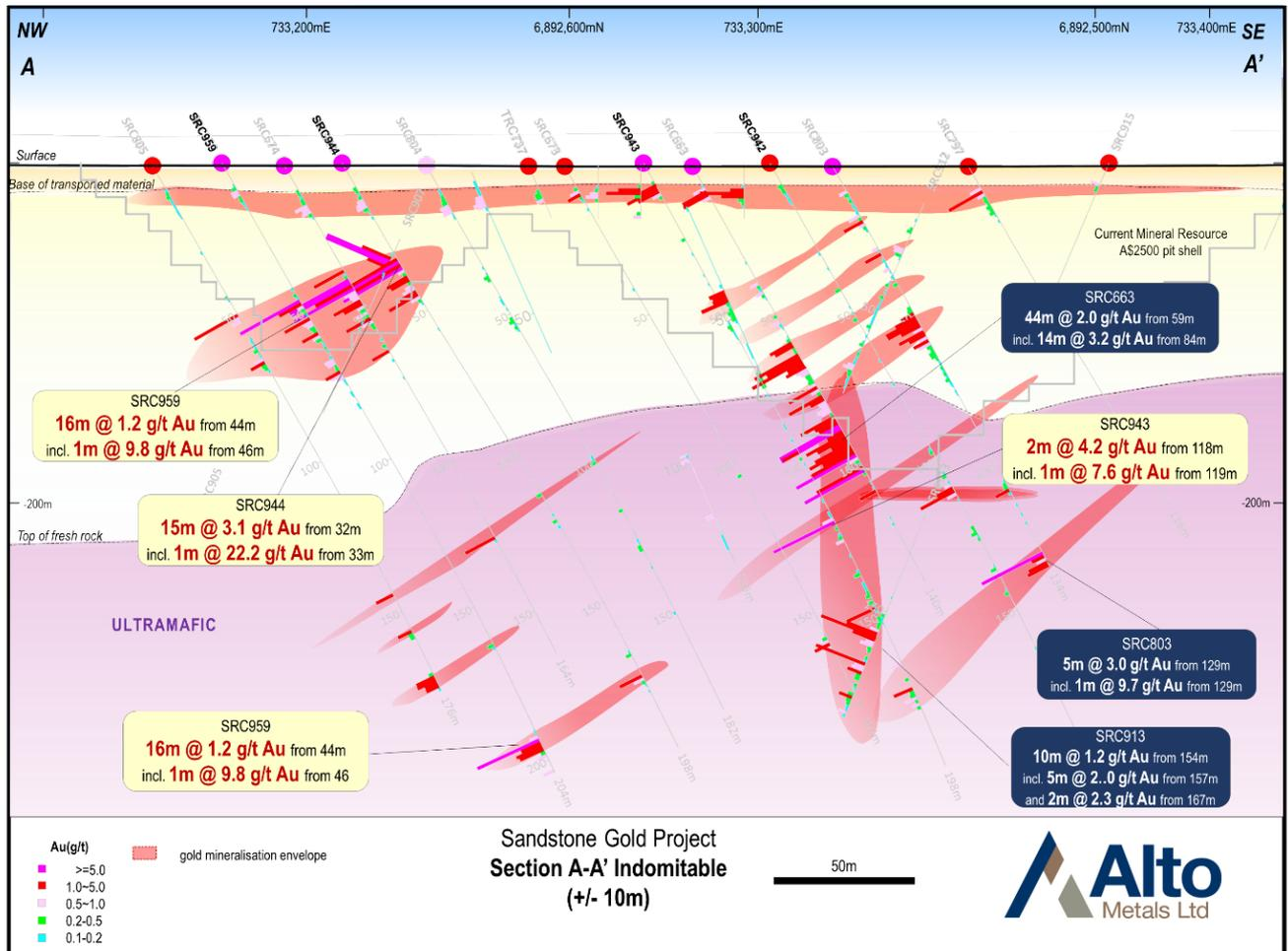
Figure 1: Indomitabile section A – A'
