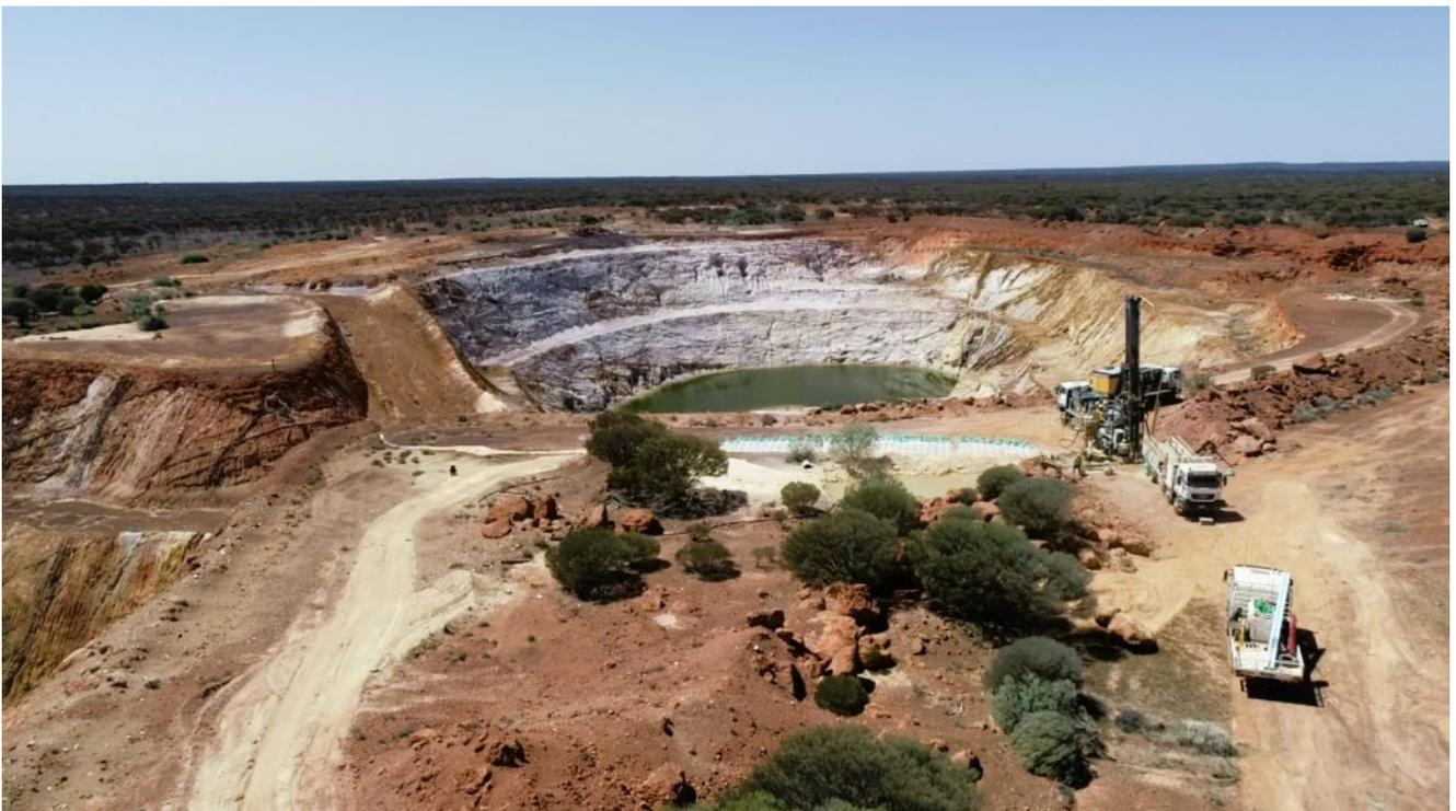
**Figure 13.** RC drilling at Bull Oak, Sandstone Gold Project.
