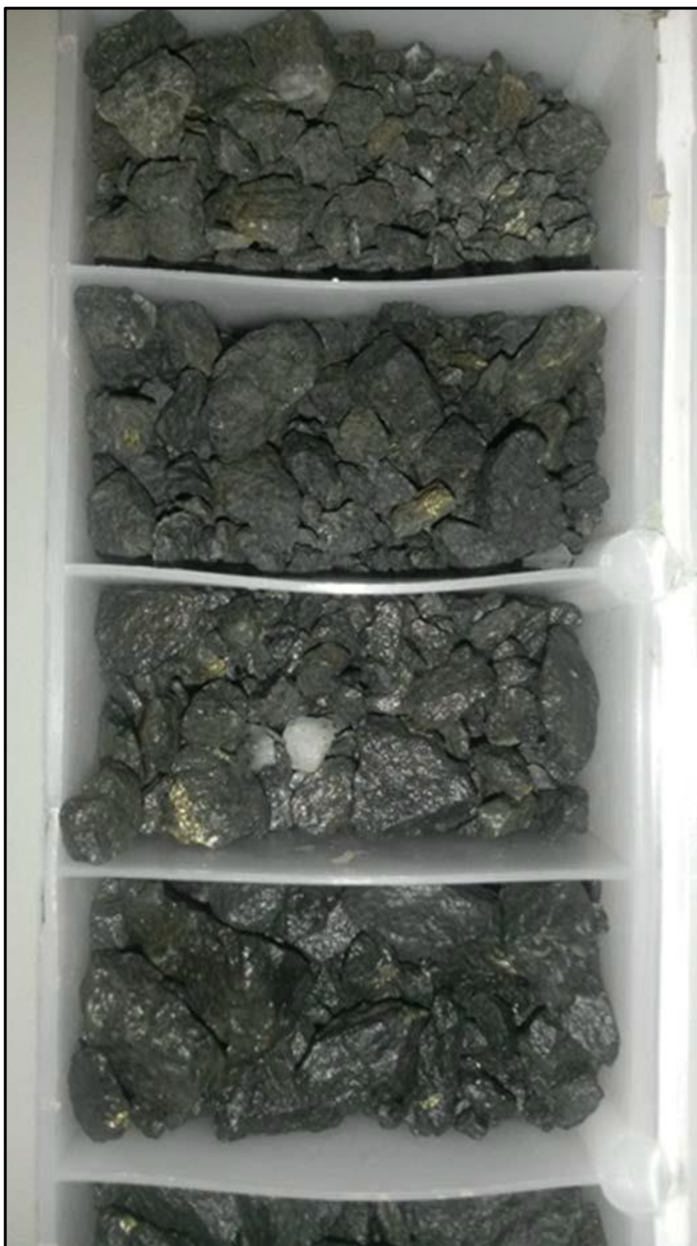
Plate 2. Drill Chips Hole SRC016: 4m @ 7.2g/t Au from 132m - 136m
