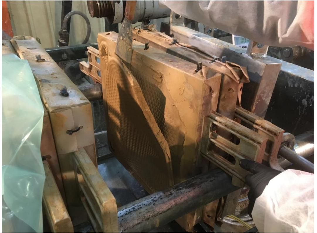
Removing Pre-Leach Residue from Filter Press
