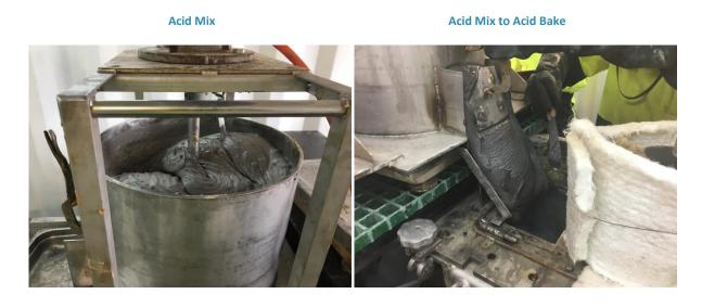
Mixing During Acid Bake Showing Visible Paddles
