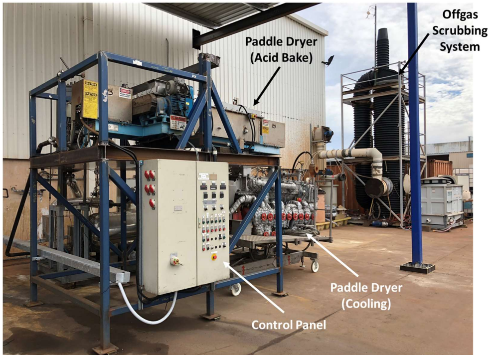
Figure 3: Phase 4 Acid Bake Pilot Plant at SGS Awaiting Installation of PLR Feeder and Pug Mixer
