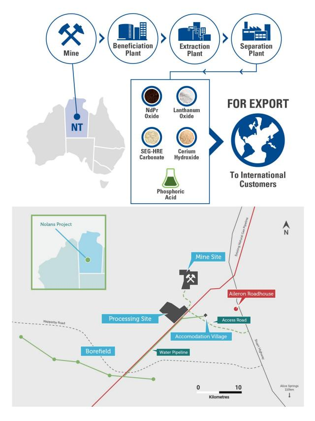
Figure 1: Project Configuration (top) and General Site Layout (bottom)
