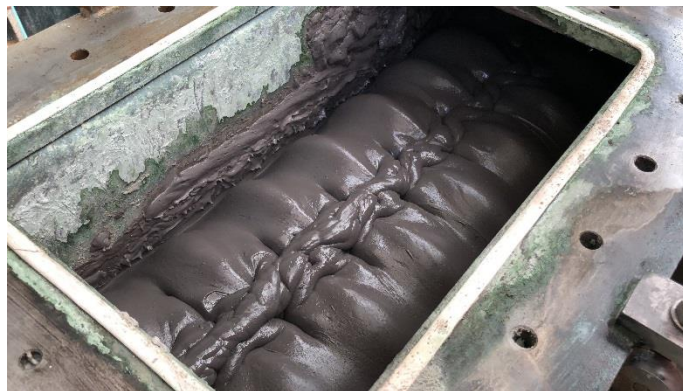
Paddle Dryer used for bake and cooling
