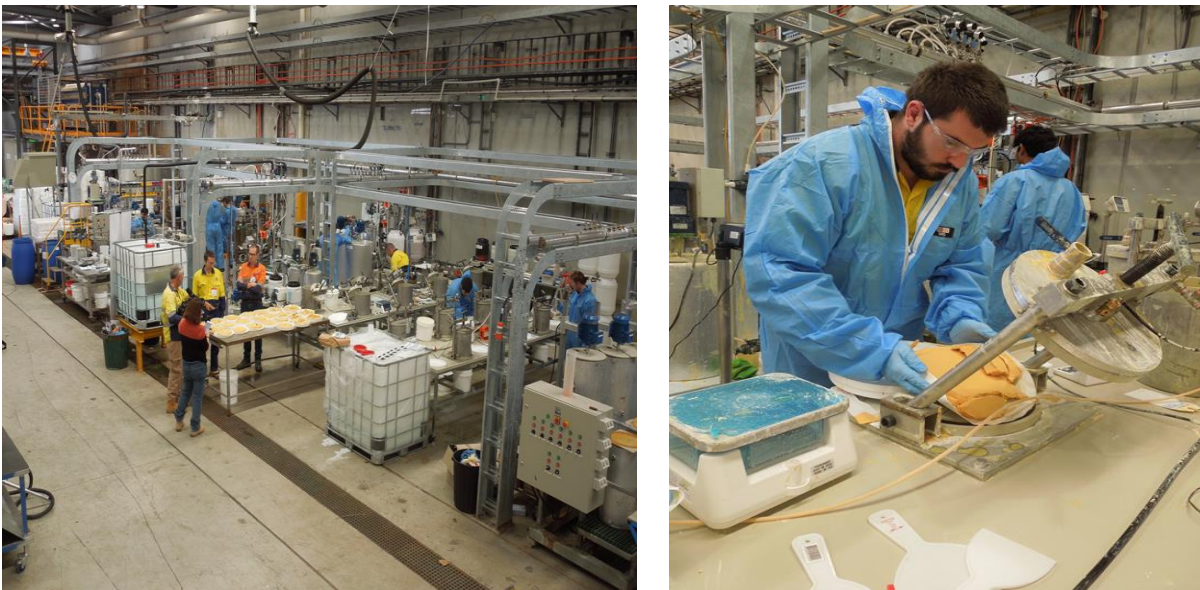
Figure 3: Phase 5 Pilot Plant (L) and Rare Earth Hydroxide Precipitate being removed from filter unit (R)
