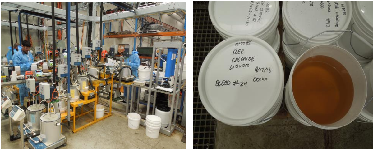
Figure 4: Phase 6 Pilot Plant Rare Earth Hydroxide Dissolution Circuit (L) and NdPr-enriched Rare Earth Chloride Liquor (R)
