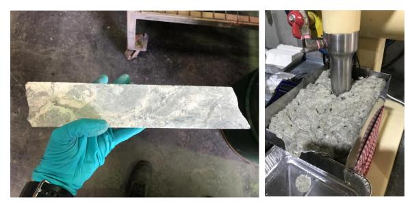
Figure 1: 5A2 drill core sample for flotation variability program (left) and flotation test (right).
