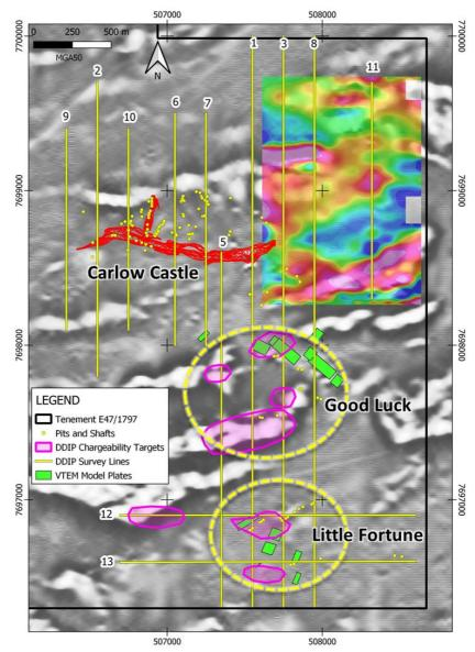
**Figure 2:** Map showing the location of Carlow Castle DDIP survey lines (yellow) and colour image of GAIP chargeability, overlying a magnetic anomaly image after 2<sup>nd</sup> vertical derivative filtering. Also shown is the Carlow Castle and Quod Est resource wire frame outline (red), historical mine workings (yellow dots), DDIP chargeability target outlines (purple), and modelled VTEM airborne electromagnetic conductor source targets (green rectangles).
