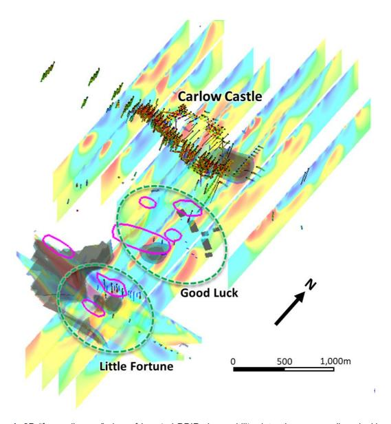
**Figure 4:** 3D "fence diagram" view of inverted DDIP chargeability data along survey lines looking to the northwest from above. Also shown are 3D bodies of high chargeability zones (grey), chargeability target outlines (purple), modelled VTEM electrical conductor source bodies (grey rectangles), and drillhole traces with elevated Cu assays plotted as hot colours downhole where historical assay data were available.
