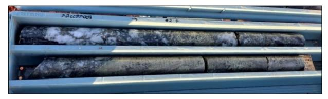
Figure 6: 22CCRD008 (256.3-258m) – Semi massive – massive sulphide in sub vertical (apparent NWN striking) vein. The is the upper zone of sulphide occurrence in the same hole.
