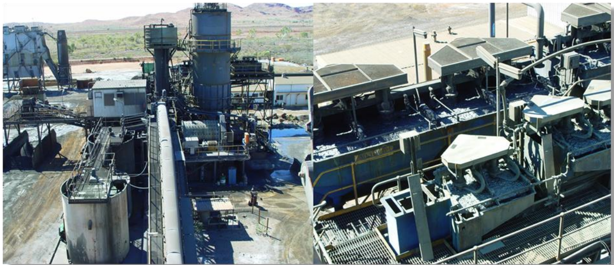
Figure 2: AGIP Radio Hill Nickel/Copper Operations (Fox 100%) - Radio Hill 425,000 tpa Treatment Plant and floatation circuits.
