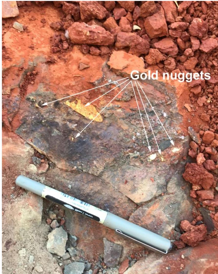
Figure 1: Coarse gold nuggets exposed in conglomerate bedrock on the floor of the first trial test trench at the Purdy's Reward prospect. The largest nugget is 4 cm long and is water worn indicating a paleo-alluvial origin.
