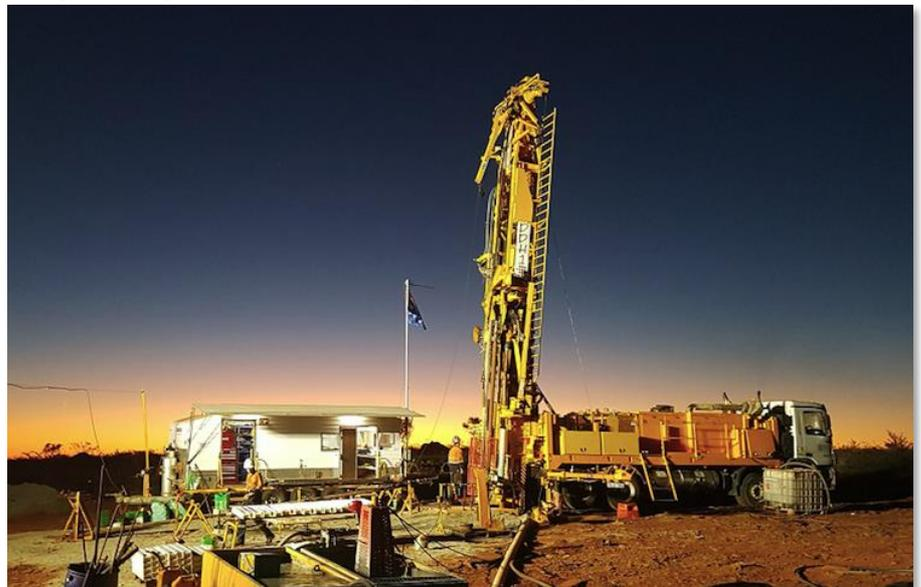
ASD-1 is planned for a vertical depth of +3,300m and designed to test the many rock sequences in the Pilbara Basin from surface and deep into the basement’s geology. DDH1 Drilling Pty Ltd ([www.ddh1.com.au](http://www.ddh1.com.au)), specialists in deep diamond drilling, is contracted to drill this hole for Artemis.
