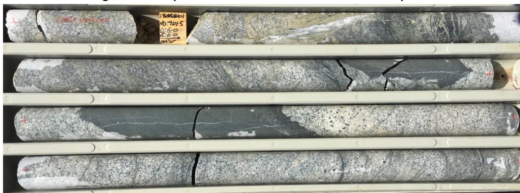
Figure 1: Core photo from ASD-1 at circa 900 metres depth.
