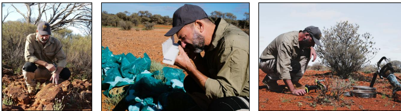
Figure 6: Asra's Exploration Manager at Yttria inspecting drill chips and taking Niton pXRF readings of soil samples.
