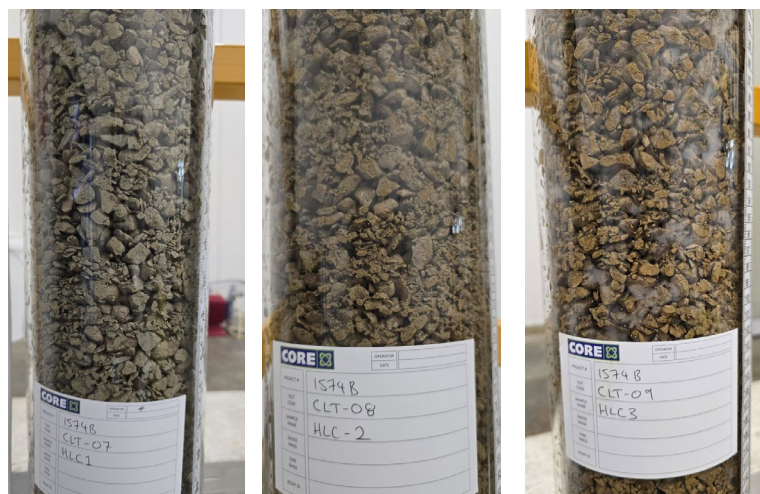
CORE Resources has been undertaking column leach testwork as part of the ongoing heap leach approach.
