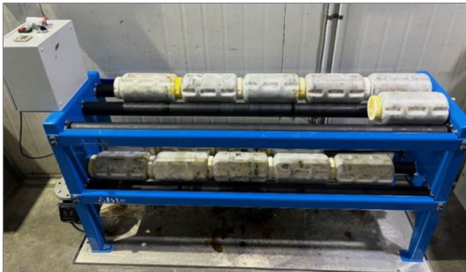
Figure 2.9: Dubbo Project – Phase 2 bottle roll leach test set-up
