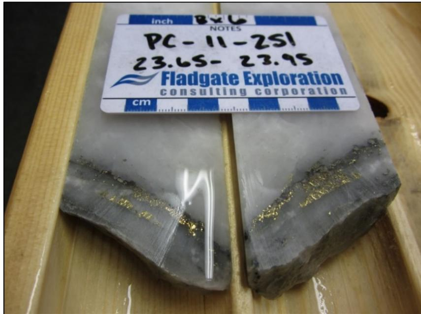
*Figure 1: Vein 22: Close up of Interval Outside of Resource Estimate. PC-11-251: Detail of interval grading 0.5m @ 1325.73g/t gold from 23.65m.*
